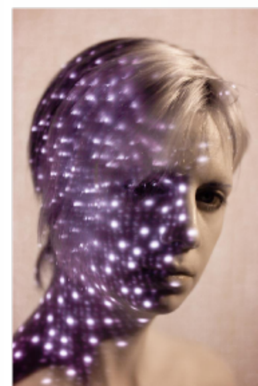
(Below) The Kinect sensor projects a structured light grid, which it uses to calculate the depth field, onto the face of a model. In normal lighting conditions this grid is invisible.
